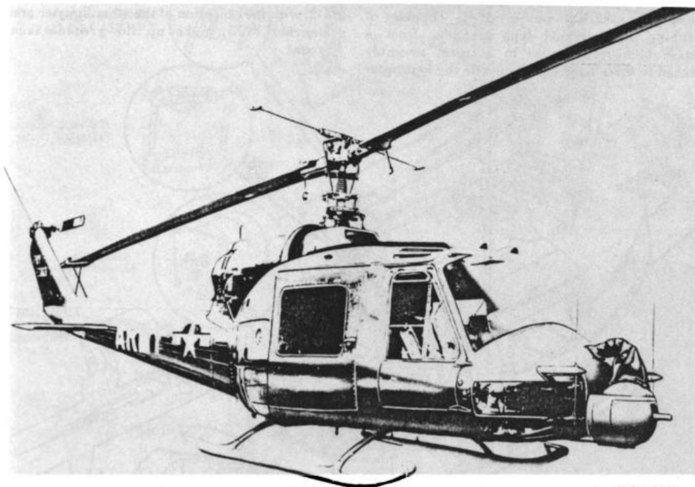
Figure 1-1. 40 Millimeter grenade launcher helicopter armament subsystem M5 installed on UH-1B helicopter—right front view.
