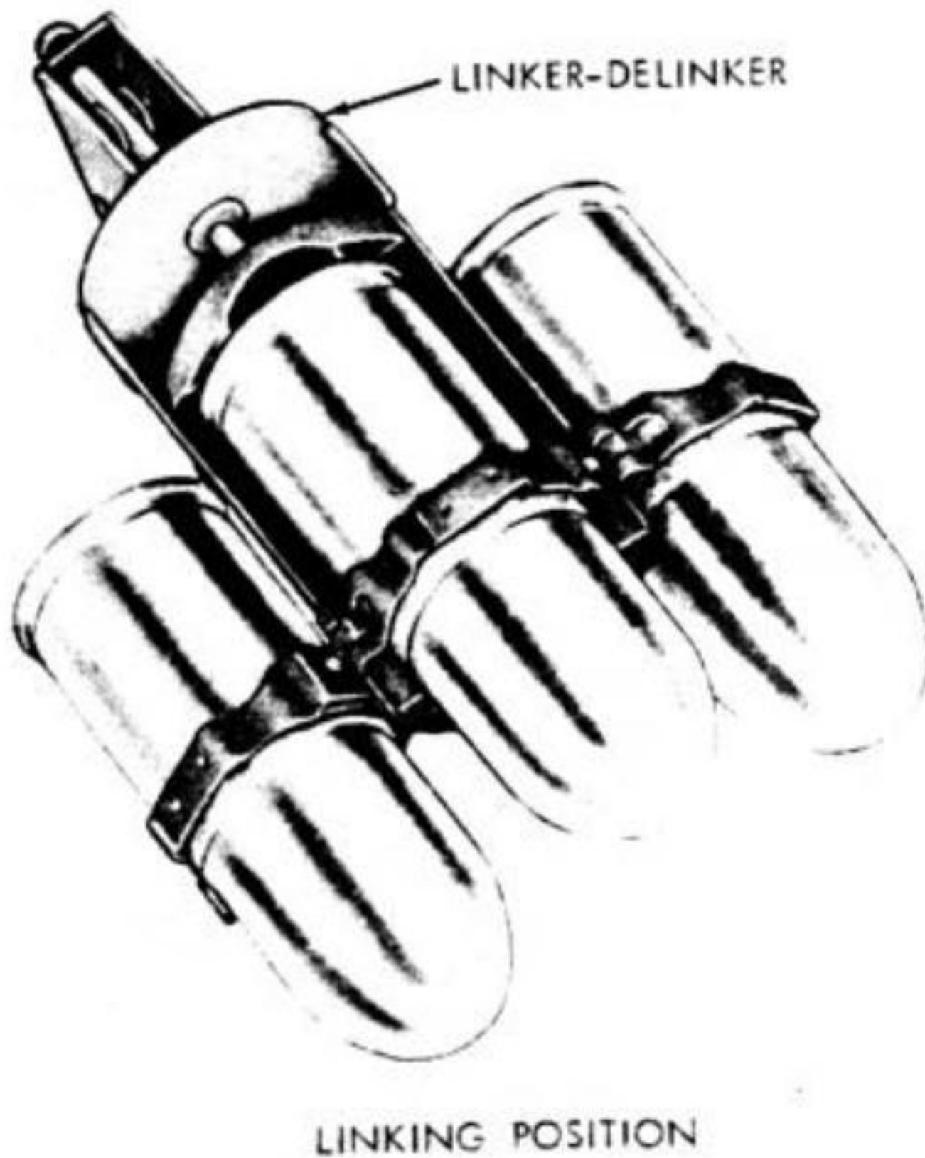
Figure 2-22. Use of hand linker-delinker.
